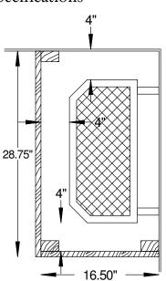
Figure 6. FHSH heater guard specifications
