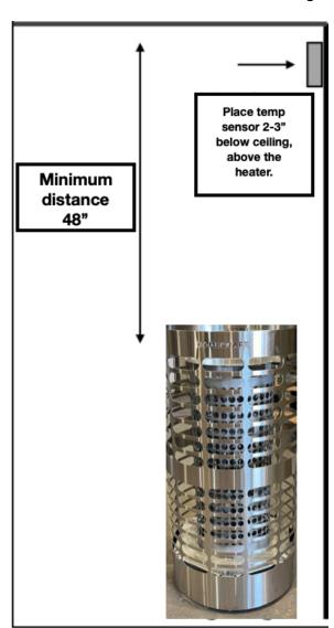
NOTE: ALL HOMECRAFT HEATERS SHOULD BE INSTALLED BY A CERTIFIED OR QUALIFIED ELECTRICIAN & IN ACCORDANCE TO LOCAL REGULATIONS
