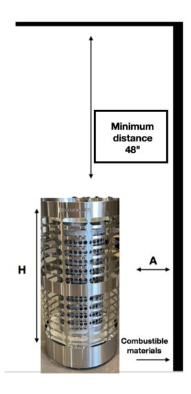
It is important to recheck your safety to combustible to ensure you have the correct safety spacing
